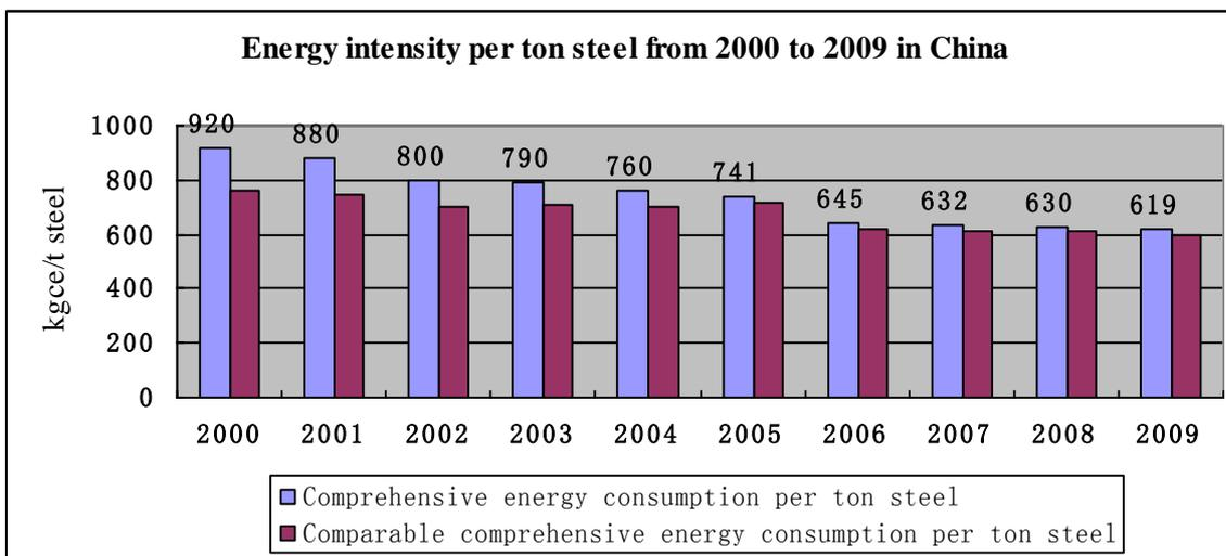
**Figure 3.5 Changes of comprehensive energy consumption<sup>2</sup> and comparable energy consumption<sup>3</sup> of major steel enterprises in China.**
