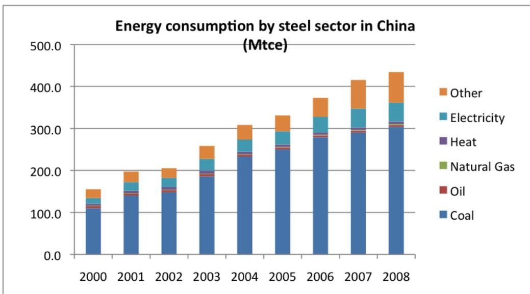
Figure 3.4 Energy consumption changes in I&S industry from 2000 to 2008
