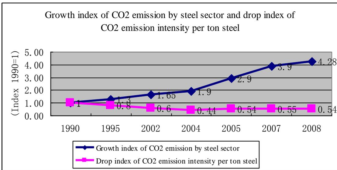
**Figure 3.6 CO<sub>2</sub> emission growth index and per ton carbon intensity drop index of China's Steel Industry from 1990 to 2008**
